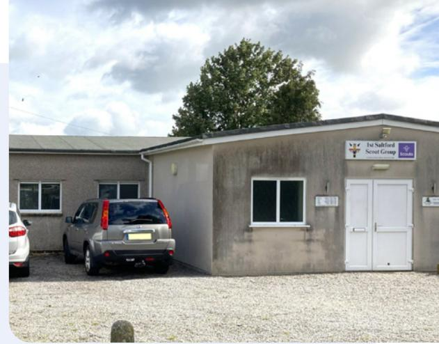
The Saltford Scout Group had a difficult building to retrofit and limited funds to address the energy and heat inefficiencies – the hut is a 1950s build with a curved roof, solid concrete walls and no insulation, making it difficult to keep both warm and cool.
